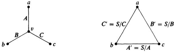
Figure II.4. The star-delta transformation;  $S = AB + BC + CA$ .
