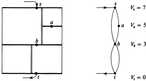
Figure II.7. The electrical network associated with our rectangle.
