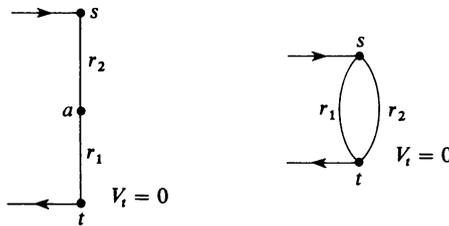
Figure II.2. Resistors connected in series and in parallel.
