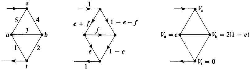
Figure II.1. The resistances, the currents and the potentials.
