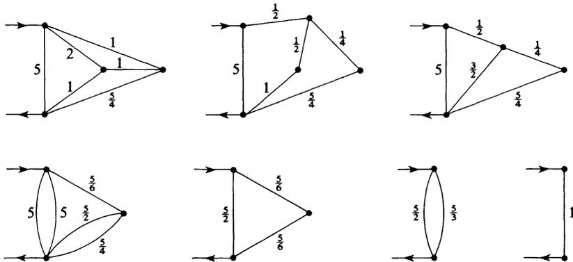
Figure II.5. Applications of the star-delta transformation.
