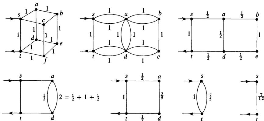
Figure II.3. Calculating the total resistance of a cube.
