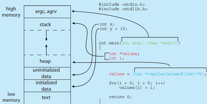
The GNU `size` command can be used to determine the size (in bytes) of some of these sections. Assuming the name of the executable file of the above C program is `memory`, the following is the output generated by entering the command `size memory`:
