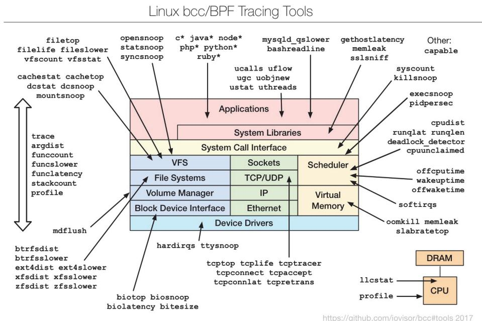
Figure 2.20 The BCC and eBPF tracing tools.
