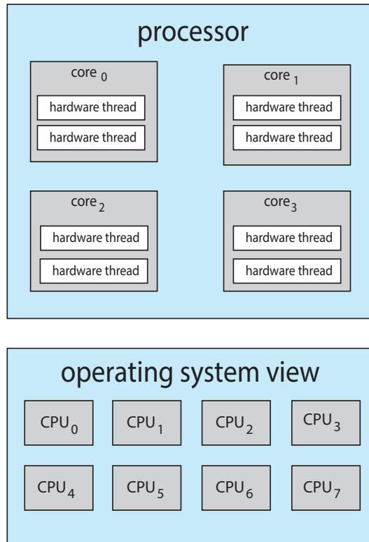
Figure 5.14 Chip multithreading.
