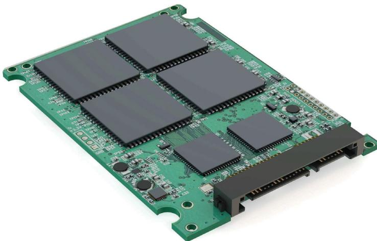
**Figure 11.3** A 3.5-inch SSD circuit board.
