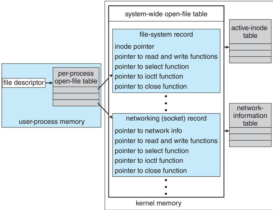
Figure 12.13 UNIX I/O kernel structure.
