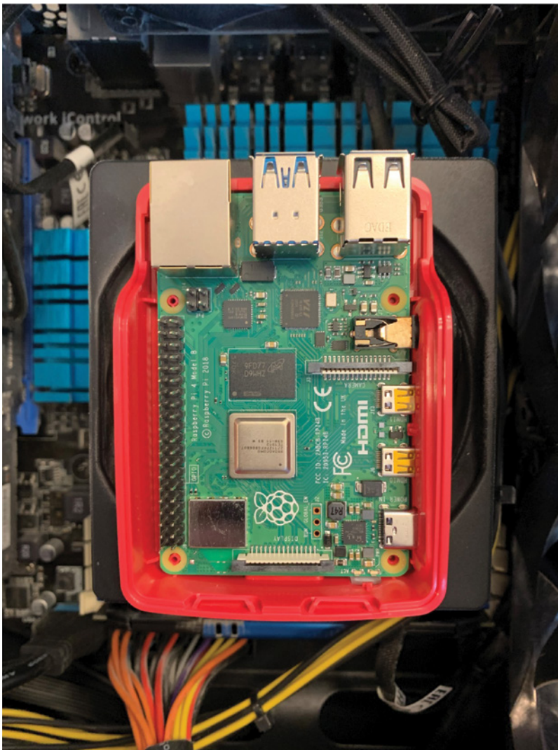
FIGURE 13.8: Raspberry Pi compared with a traditional processor
