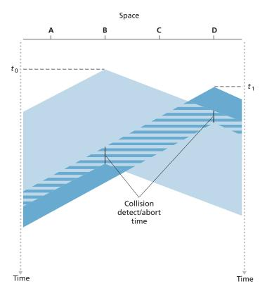
Figure 6.13 ◆ CSMA with collision detection
