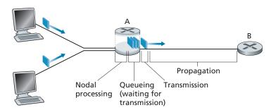
Figure 1.16 → The nodal delay at router A
