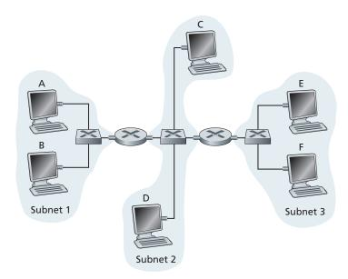
Figure 6.33 ◆ Three subnets, interconnected by routers
