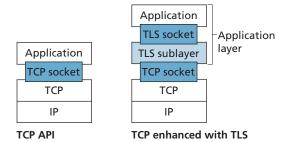
Figure 8.24 • Although TLS technically resides in the application layer, from the developer's perspective it is a transport-layer protocol
