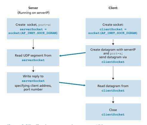
Figure 2.27 ◆ The client-server application using UDP
