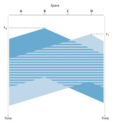
Figure 6.12 • Space-time diagram of two CSMA nodes with colliding transmissions
