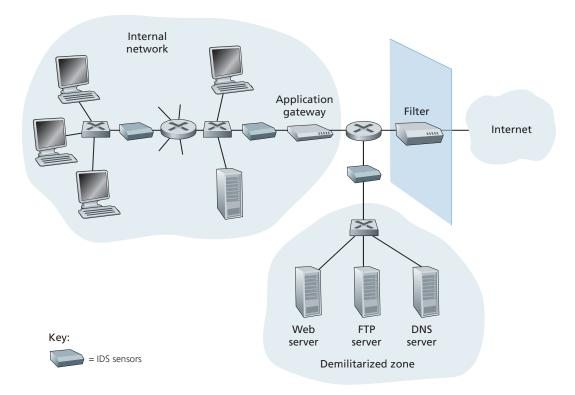
Figure 8.37 • An organization deploying a filter, an application gateway, and IDS sensors
