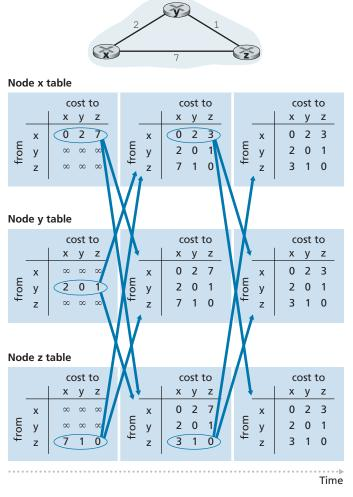
Figure 5.6 → Distance-vector (DV) algorithm in operation
