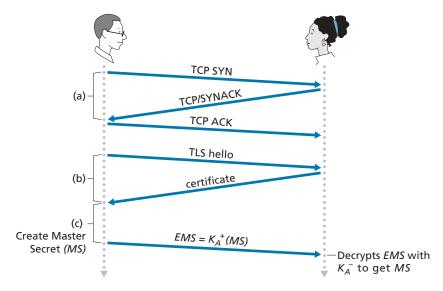
Figure 8.25 • The almost-TLS handshake, beginning with a TCP connection
