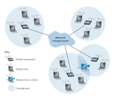
Figure 7.1 → Elements of a wireless network
