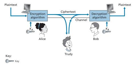
Figure 8.2 ◆ Cryptographic components
