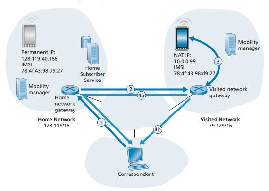
Figure 7.26 + Indirect routing to a mobile device
