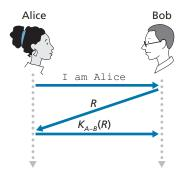
**Figure 8.18** ◆ Protocol ap4.0 and a failure scenario
