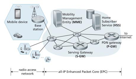
Figure 7.17 → Elements of the 4G LTE architecture
