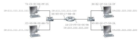
Figure 6.19 ◆ Two subnets interconnected by a router
