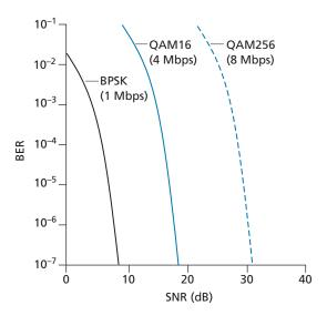
Figure 7.3 ◆ Bit error rate, transmission rate, and SNR
