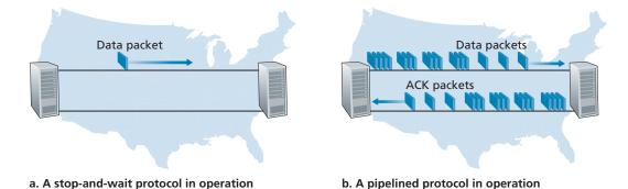
Figure 3.17 ◆ Stop-and-wait versus pipelined protocol
