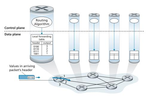
Figure 4.2 ◆ Routing algorithms determine values in forward tables
