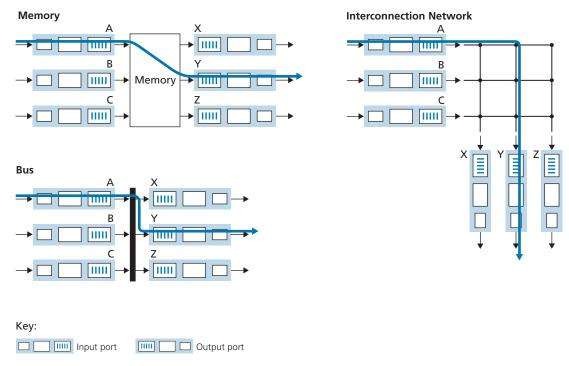
Figure 4.6 ◆ Three switching techniques
