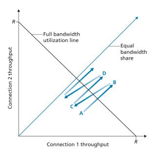
Figure 3.57 → Throughput realized by TCP connections 1 and 2
