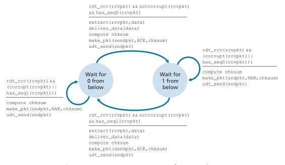
Figure 3.60 • An incorrect receiver for protocol rdt 2.1
