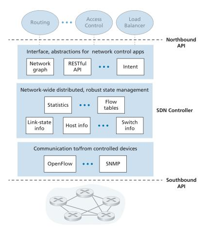
Figure 5.15 → Components of an SDN controller
