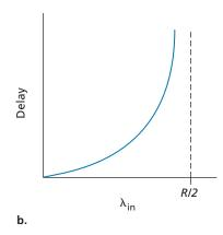
Figure 3.44 • Congestion scenario 1: Throughput and delay as a function of host sending rate
