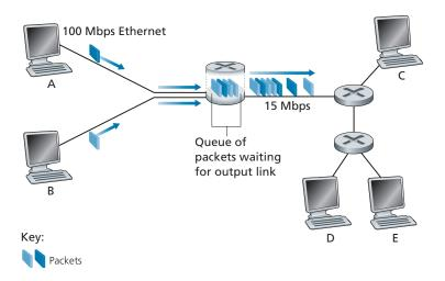
Figure 1.12 ◆ Packet switching
