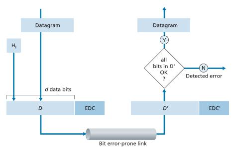
Figure 6.3 ◆ Error-detection and -correction scenario
