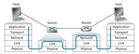
Figure 6.24 ◆ Packet processing in switches, routers, and hosts
