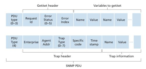
Figure 5.21 ◆ SNMP PDU format
