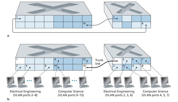
Figure 6.26 • Connecting two VLAN switches with two VLANs:
