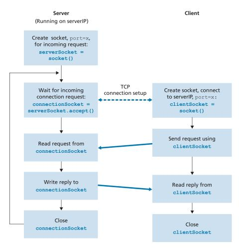
Figure 2.29 ◆ The client-server application using TCP
