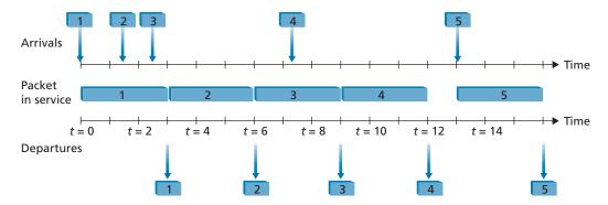
Figure 4.12 → The FIFO queue in operation
