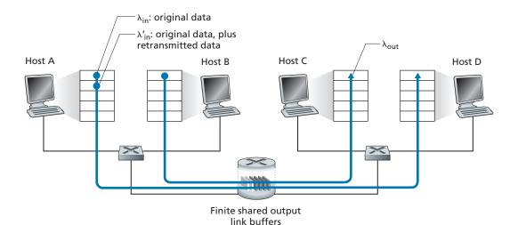
Figure 3.45 • Scenario 2: Two hosts (with retransmissions) and a router with finite buffers
