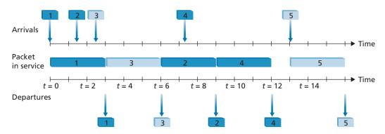
Figure 4.15 ◆ The two-class robin queue in operation
