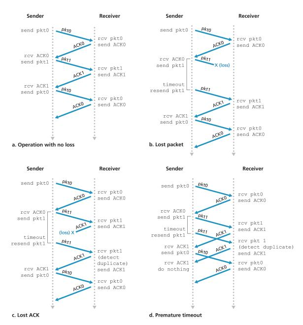
Figure 3.16 • Operation of rdt3.0, the alternating-bit protocol
