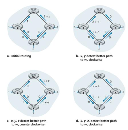
Figure 5.5 ◆ Oscillations with congestion-sensitive routing
