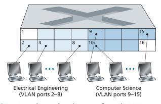
**Figure 6.25 →** A single switch with two configured VLANs
