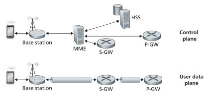
Figure 7.18 → LTE data-plane and control-plane elements
