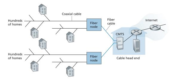
Figure 1.6 ◆ A hybrid fiber-coaxial access network
