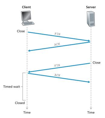
Figure 3.40 → Closing a TCP connection
