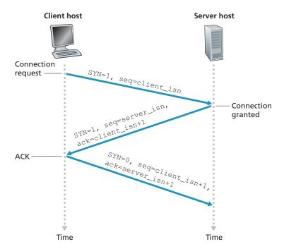
Figure 3.39 ◆ TCP three-way handshake: segment exchange
