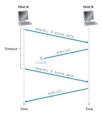
Figure 3.34 ◆ Retransmission due to a lost acknowledgment
