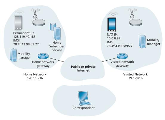
Figure 7.25 → Elements of a mobile network architecture
