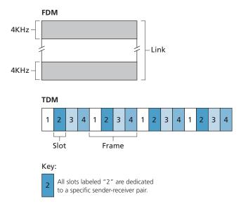
Figure 6.9 • A four-node TDM and FDM example
