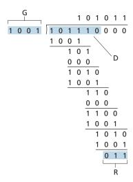
Figure 6.7 ◆ A sample CRC calculation
