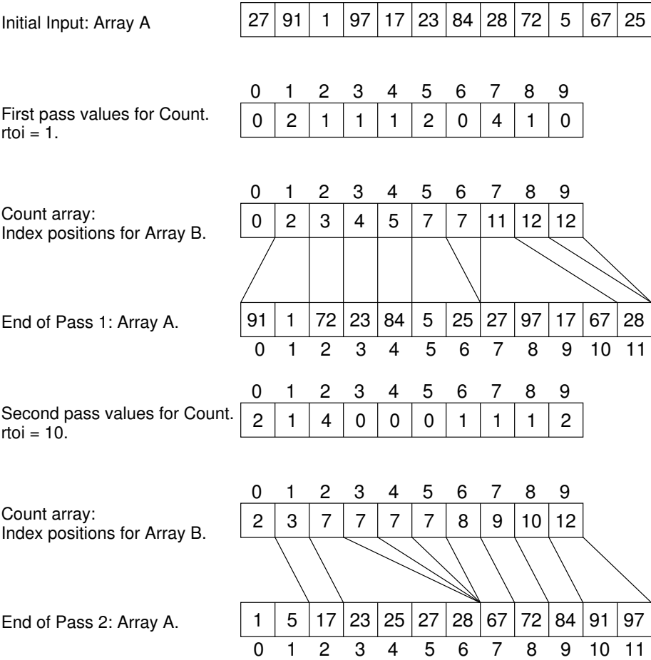
Figure 7.19 An example showing function radix applied to the input of Figure 7.17. Row 1 shows the initial values within the input array. Row 2 shows the values for array cnt after counting the number of records for each bin. Row 3 shows the index values stored in array cnt . For example, cnt [0] is 0, indicating no input values are in bin 0. Cnt [1] is 2, indicating that array B positions 0 and 1 will hold the values for bin 1. Cnt [2] is 3, indicating that array B position 2 will hold the (single) value for bin 2. Cnt [7] is 11, indicating that array B positions 7 through 10 will hold the four values for bin 7. Row 4 shows the results of the first pass of the Radix Sort. Rows 5 through 7 show the equivalent steps for the second pass.
