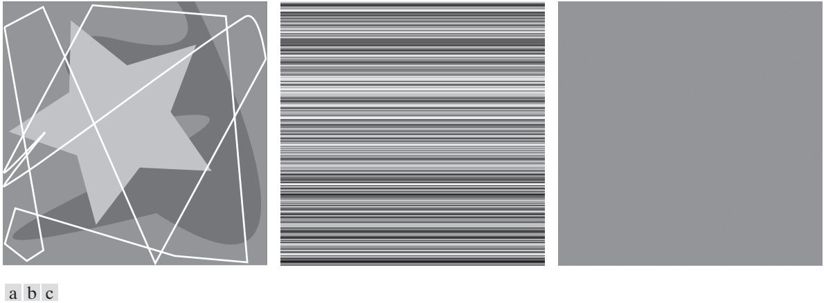
FIGURE 8.1 Computer generated 256 \times 256 \times 8 bit images with (a) coding redundancy, (b) spatial redundancy, and (c) irrelevant information. (Each was designed to demonstrate one principal redundancy, but may exhibit others as well.)
