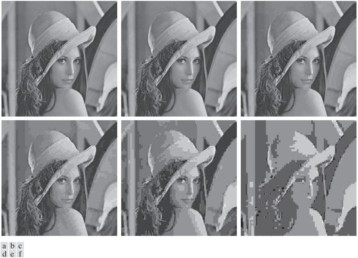
FIGURE 8.28 Approximations of Fig. 8.9(a) using the DCT and normalization array of Fig. 8.27(b): (a) Z , (b) 2Z , (c) 4Z , (d) 8Z , (e) 16Z , and (f) 32Z .
