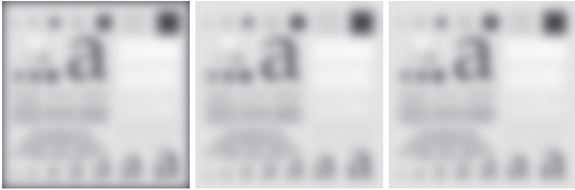
FIGURE 3.39 Result of filtering the test pattern in Fig. 3.36(a) using (a) zero padding, (b) mirror padding, and (c) replicate padding. A Gaussian kernel of size 187 \times 187 , with K = 1 and \sigma = 31 was used in all three cases.
