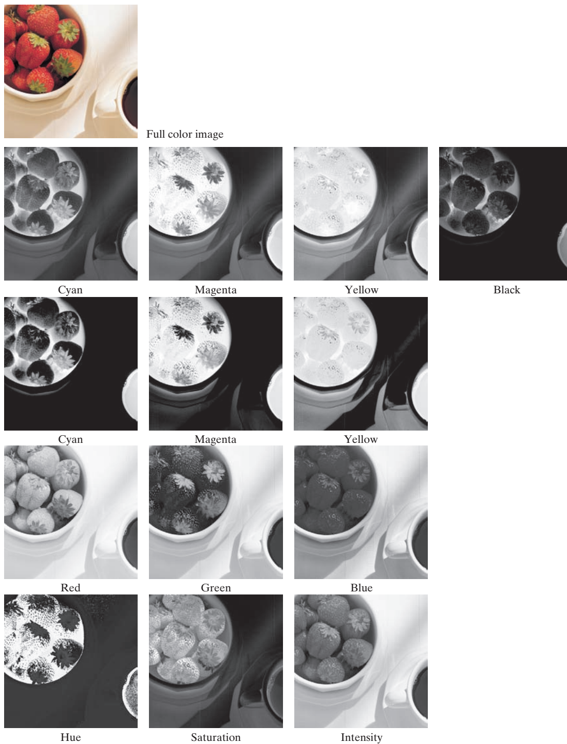
FIGURE 6.28 A full-color image and its various color-space components. (Original image courtesy of MedData Interactive.)
