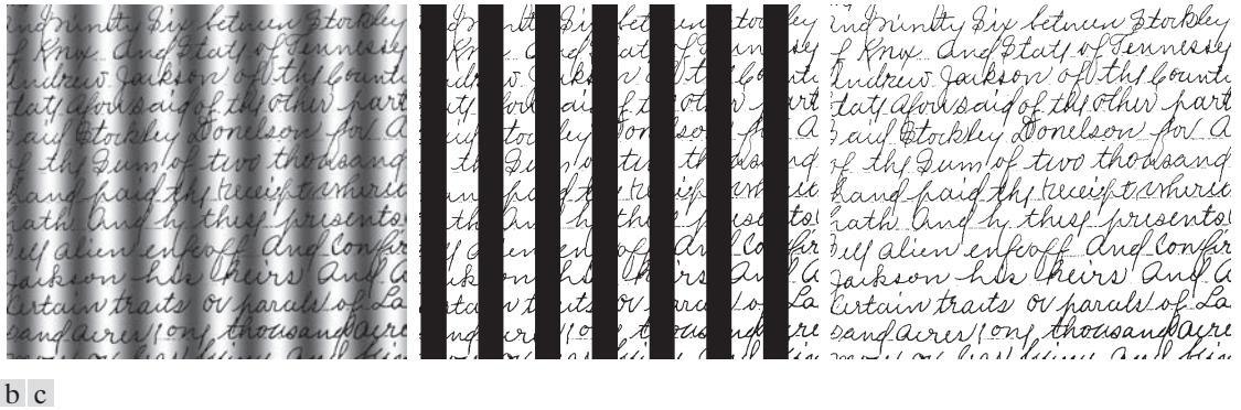
FIGURE 10.45 (a) Text image corrupted by sinusoidal shading. (b) Result of global thresholding using Otsu's method. (c) Result of local thresholding using moving averages.
