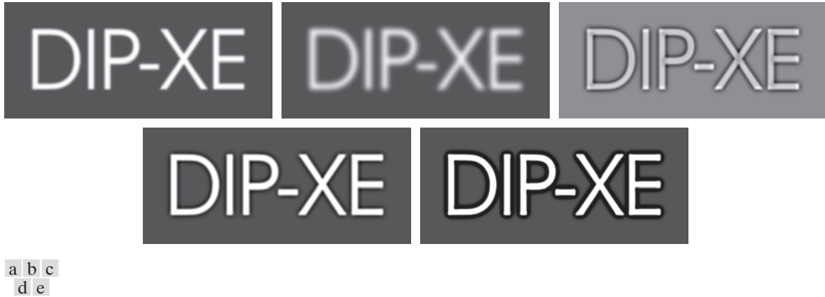
FIGURE 3.49 (a) Original image of size 600 \times 259 pixels. (b) Image blurred using a 31 \times 31 Gaussian lowpass filter with \sigma = 5 . (c) Mask. (d) Result of unsharp masking using Eq. (3-56) with k = 1 . (e) Result of highboost filtering with k = 4.5 .
