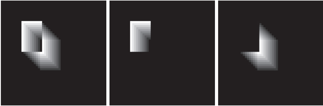
FIGURE 10.62 ADIs of a rectangular object moving in a southeasterly direction. (a) Absolute ADI. (b) Positive ADI. (c) Negative ADI.
