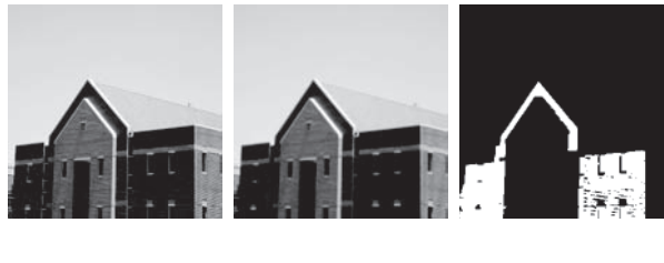
FIGURE 11.55 (a) Building image reduced to half-size. (b) Image smoothed with a 3 \times 3 box kernel. (c) Composite MSER obtained with the same parameters as Fig. 11.53(e), but using a valid MSER region size range of 2,500–7,500 pixels.
