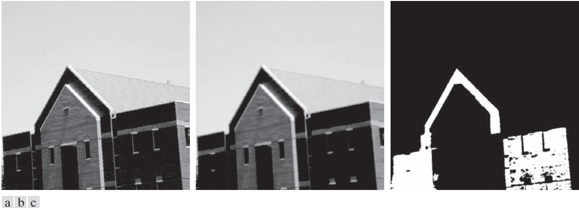
FIGURE 11.54 (a) Building image rotated 5^\circ counterclockwise. (b) Smoothed image using the same kernel as in Fig. 11.53(b). (c) Composite MSER detected using the same parameters we used to obtain Fig. 11.53(e). The MSERs of the original and rotated images are almost identical.
