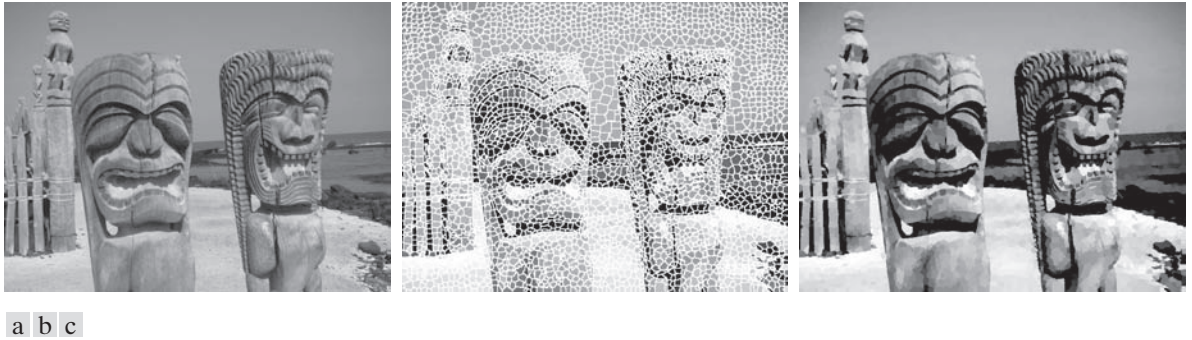
FIGURE 10.50 (a) Image of size 600 \times 480 (480,000) pixels. (b) Image composed of 4,000 superpixels (the boundaries between superpixels (in white) are superimposed on the superpixel image for reference—the boundaries are not part of the data). (c) Superpixel image. (Original image courtesy of the U.S. National Park Services.).
