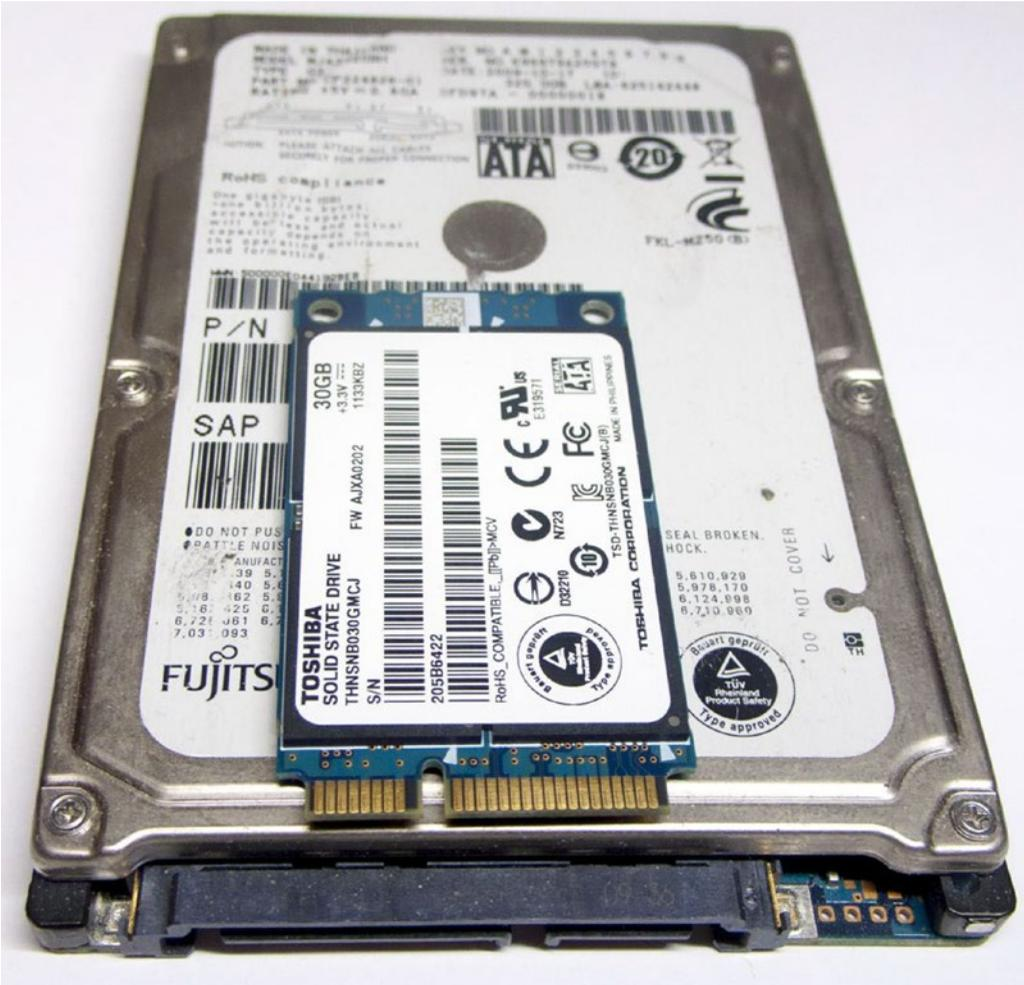
Figure 12-4. SSD drives in SATA and mSATA format<sup>2</sup>
