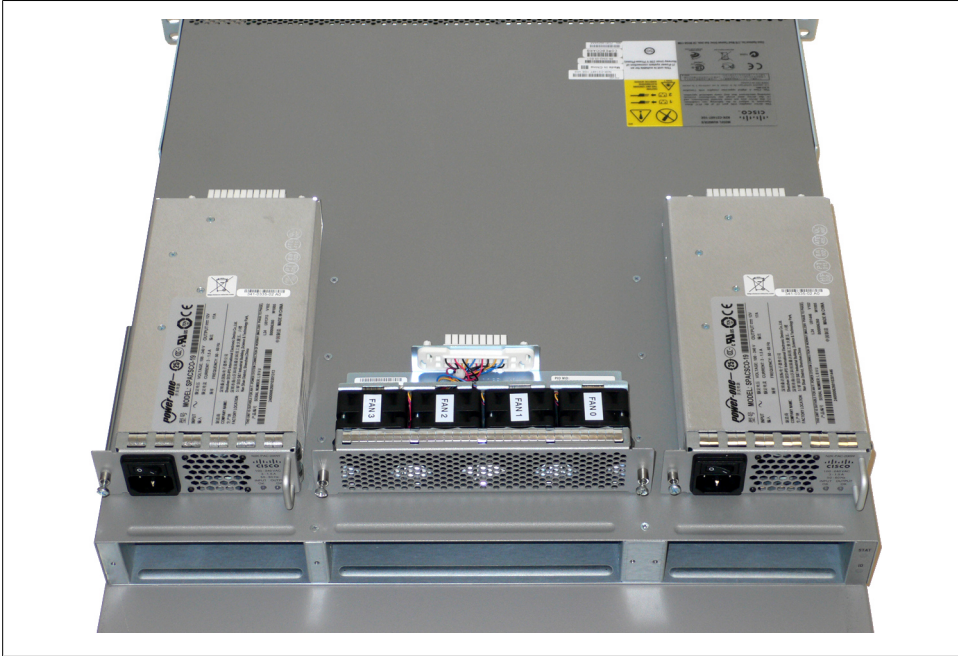
Figure 18-8. Nexus 2148 FEX with power supplies and fan tray removed
