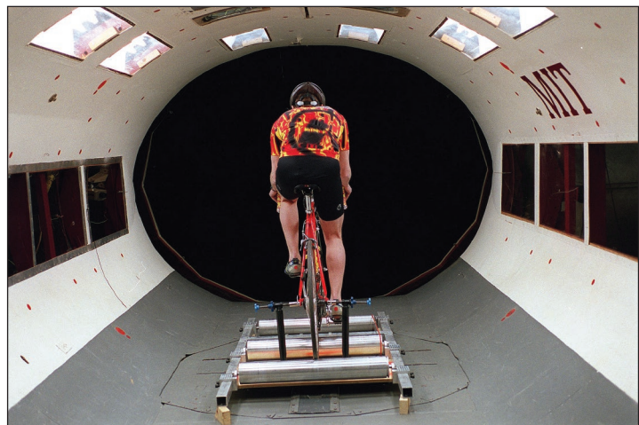
AN AERODYNAMICS EXPERT LOGS RESULTS FROM A WIND TUNNEL TEST FOR CYCLING CLOTHING AND RACING BICYCLE DESIGN.
