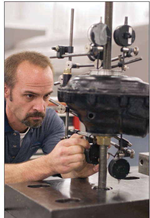
CONTROL CHECK OF A CAR AXLE AT DANA CORPORATION RESEARCH AND DEVELOPMENT CENTER.
