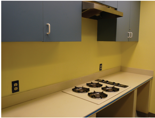
FIGURE 3.18 Corridor kitchen, D-shaped handles, lowered counter heights, space under counters for wheelchair access, side controls on the gas range.
