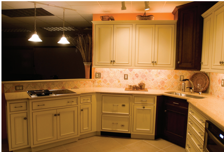
FIGURE 3.30 The floor space in the Gourmet Kitchen in the Center for Real Life Kitchen Design is large enough for a 60" turn space. At the sink, a corner wall cabinet includes a lazy Susan for more accessible storage and nearby dishwasher drawers are at a useable height.
