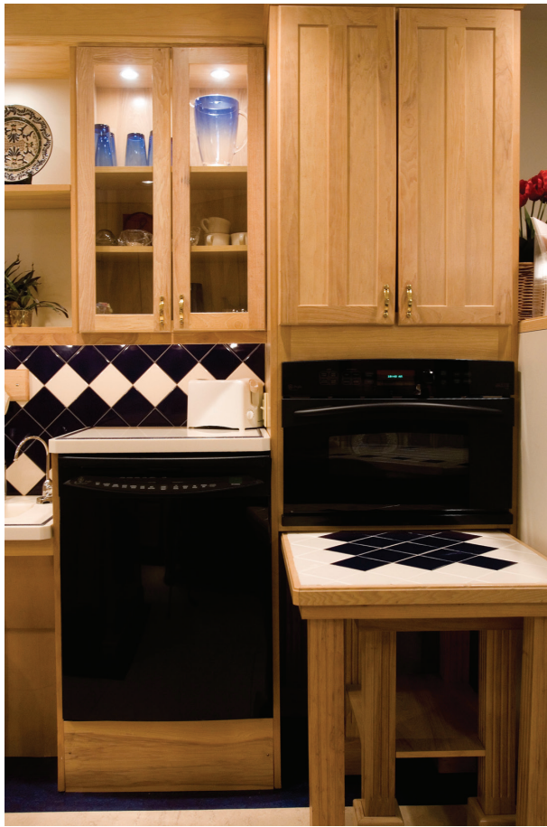
FIGURE 3.28 The raised dishwasher and the built-in speed cook oven are placed within the universal reach range. Nested carts under the oven provide a method to move food and supplies around the kitchen.
