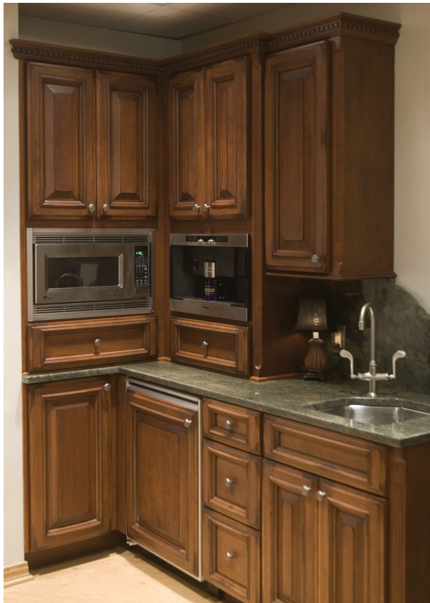
FIGURE 3.32 This small Outpost Kitchen provides a built-in microwave and coffee system within the universal reach range. The drawer under the microwave includes a shelf for a convenient landing area.
