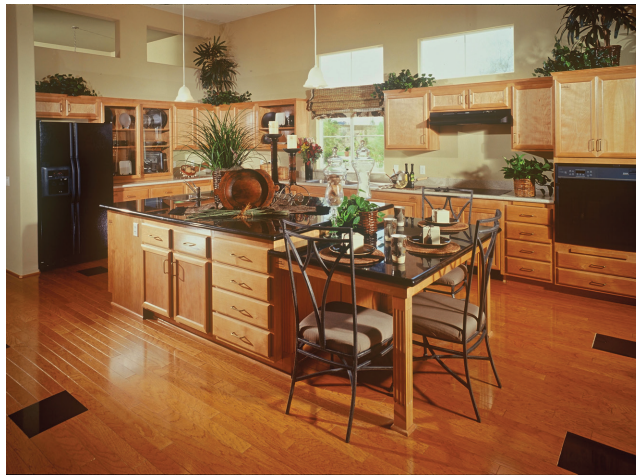
FIGURE 2.8 Flexibility in use: 48" work aisles, multiple counter heights, 48" work aisles, D-shaped pulls, a Susan Mack kitchen.
