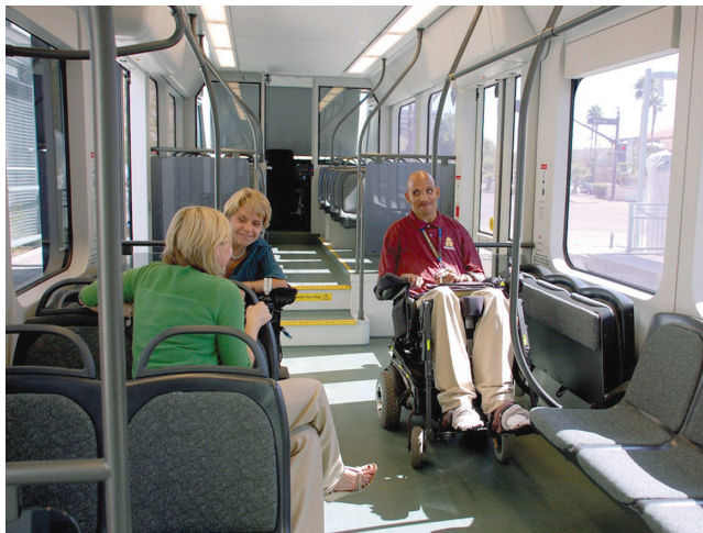
FIGURE 3.48 The Interior of the METRO vehicle allows for all riders to determine where and how they will position themselves for their trip. Bicycle riders have dedicated seating areas and hanging bike racks to accommodate their needs.
