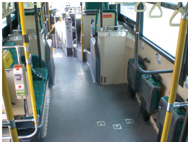
FIGURE 7.16 Three pedal-operated jump seats for passengers are sprung upward on the right side, to make space available for two wheelchair passengers. Three hooks on the floor fix a wheelchair to the floor (Kumamoto, Japan).
