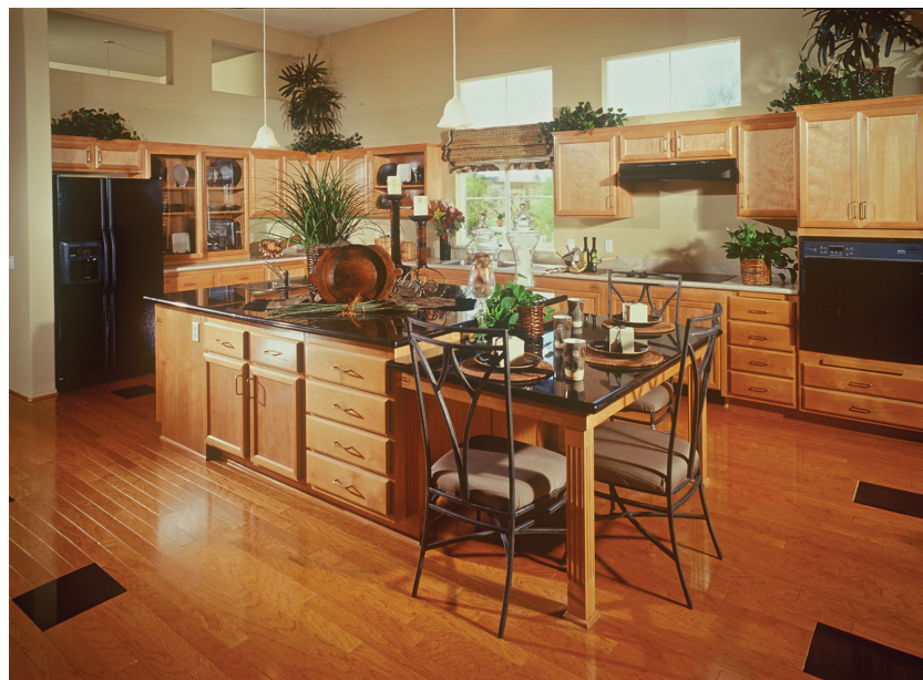
FIGURE 8.23 Accessible kitchen in Susan Mack house; multiple counter heights are shown; the side-opening oven provides easy access.
