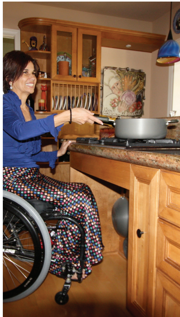
FIGURE 8.3 Valinda Martin's kitchen plates are stored vertically in the rear of the picture; her cook-top is over an open space, which not only provides storage for hanging pots, but also allows her to move into a more accessible position.
