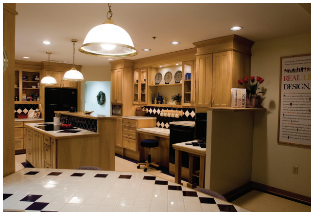
FIGURE 3.26 The GE Real Life Design Kitchen at Virginia Tech features multiple counter heights, raised toe kicks and dishwasher, under-cabinet lighting, open shelves, knee space under the sink and cooktop, carts, and contrasting floors and counter edging.
