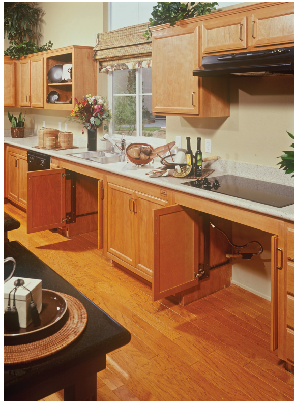
FIGURE 2.14 Size and space: knee space at sink and cooktop with retractable cabinet doors, by Susan Mack.
