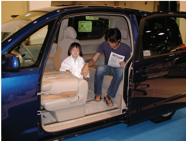
FIGURE 5.17 Open sliding driver's door revealing fold-down front seat, Toyota.
