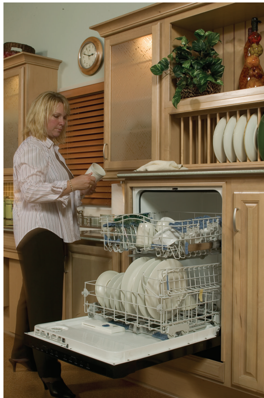
FIGURE 3.37 Kitchen with a raised dishwasher and vertical plate storage.
