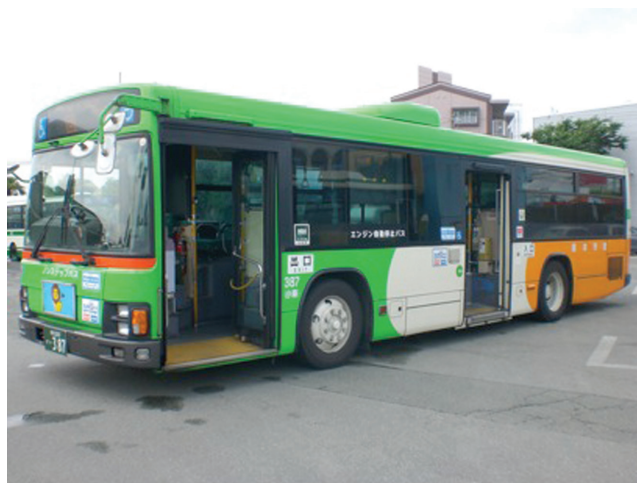
FIGURE 7.13 Outside appearance of a low-floor bus with no step barrier (Kumamoto, Japan).
