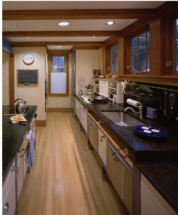
FIGURE 8.30 Kitchen in John Salman's home features a variety of counter heights and front grab bars.
