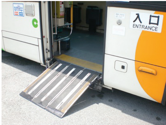
FIGURE 7.14 The movable sliding ramp is placed sloped at the bus's central entrance (Kumamoto, Japan).
