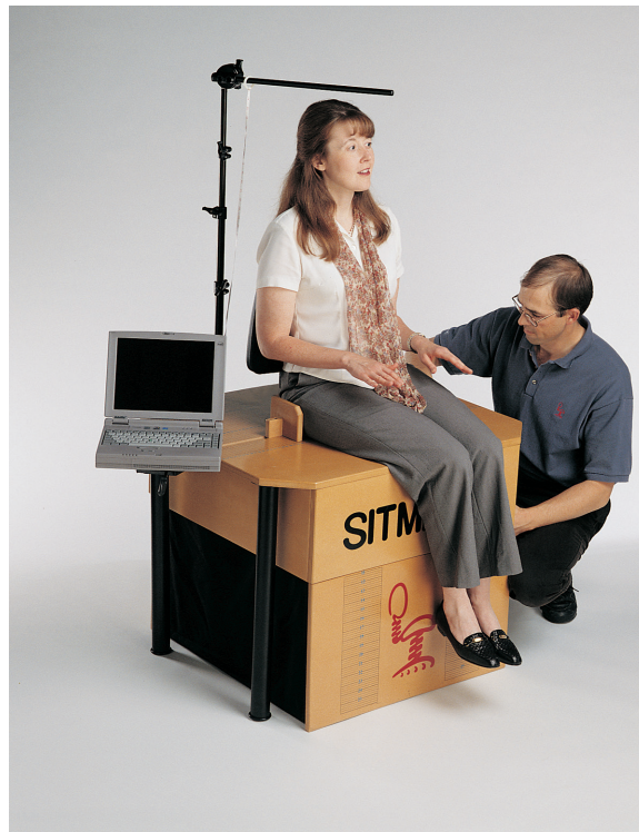
FIGURE 6.4 Sitmatic measuring device for custom chair design.
