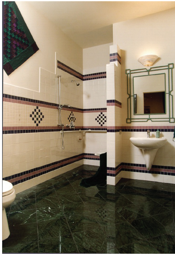
FIGURE 8.2 This bath utilizes several recommended features: color contrast, smooth floor surfaces, curbless shower with flexible water dam, grab bars, a wall-hung sink, and a raised toilet seat.
