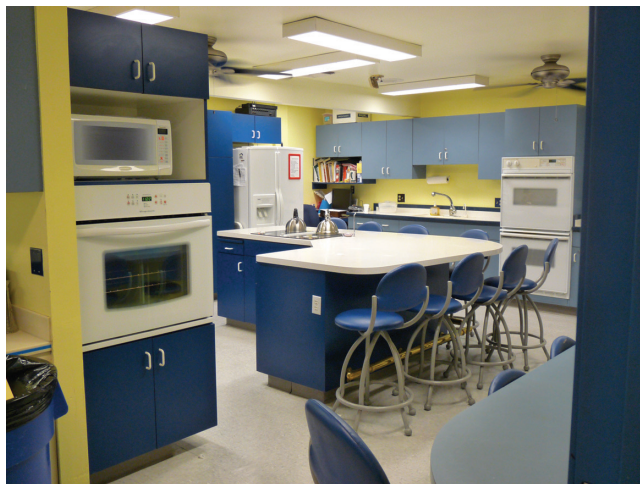
FIGURE 3.17 Kitchen features: color contrast between cabinets and countertop, sturdy Bola stools, varied height counter/cabinets, D-shaped handles on cabinets.
