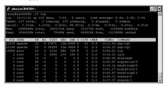
The upper part also provides loads of useful statistics on the current resource usage such as system uptime, active users, load average, memory and processor load, and more.
