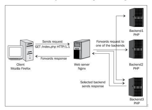
In this case, Nginx is connected to multiple backend servers. To establish such a configuration, a new module comes into play – the **Upstream module**.
